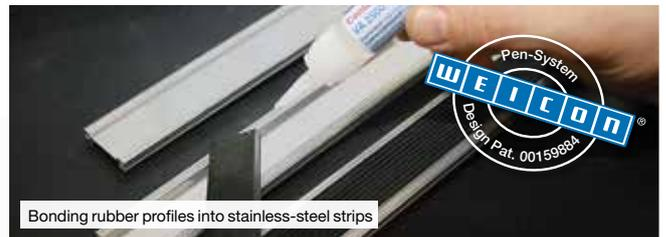
Bonding rubber profiles into stainless-steel strips
