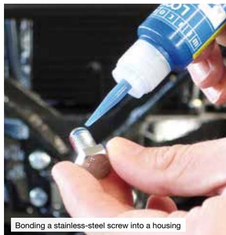
Bonding a stainless-steel screw into a housing
